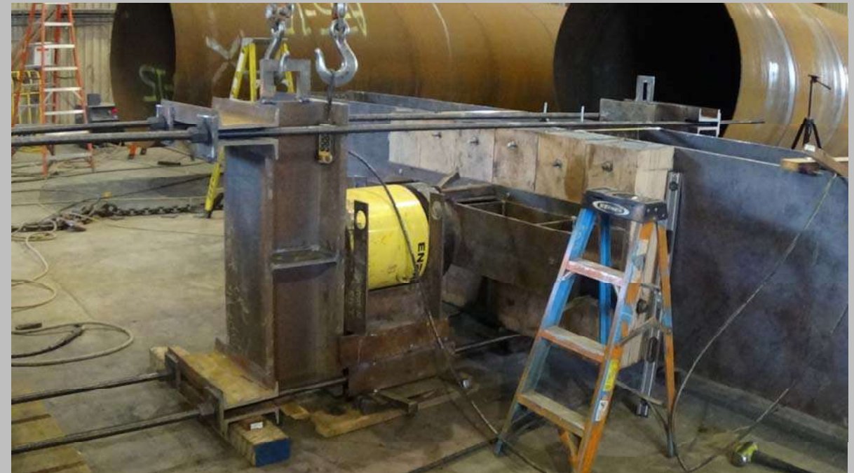
Compression “crush” Test
