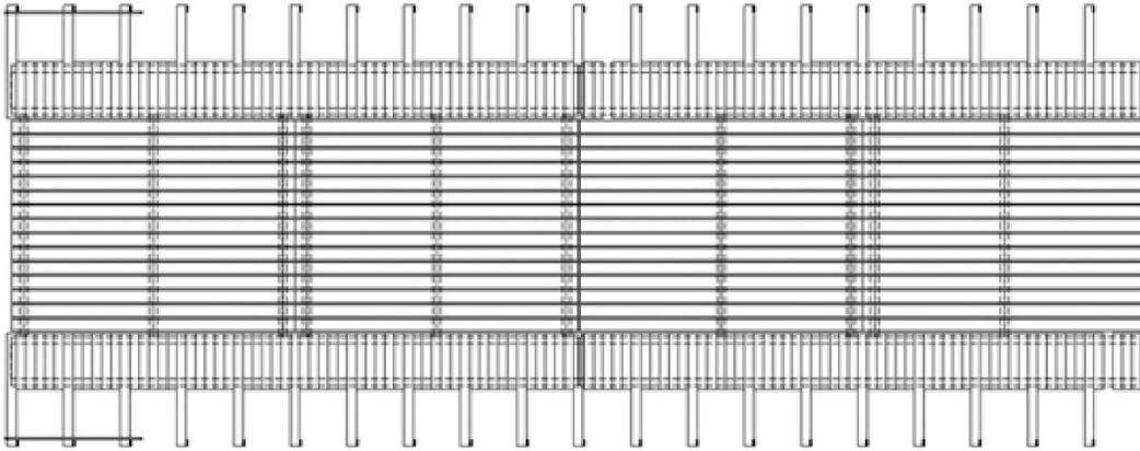
**Fig. 8 Omega Beam - perspective view & end detail**
